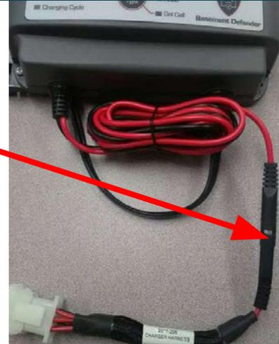
Plug Battery harness into Battery 1 connector
